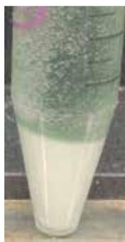
Table 4. REE enrichment into the solution and precipitate from NiMH battery waste. Figure shows the REE precipitate formed.
