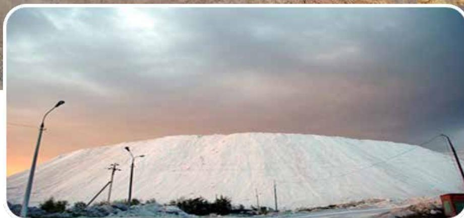
Figure 1. Jarosite and phosphogypsum heap.
