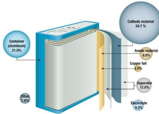
**Figure 2.** Lithium ion battery construction.
