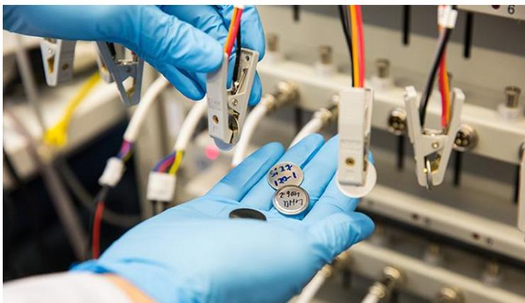
**Figure 4.** Characterization of ALD/MLD grown microbatteries. Photo by Mikko Raskinen, Aalto University.
